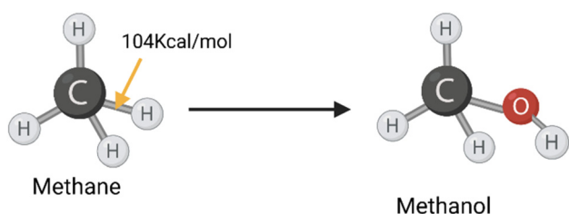
Fig. 17 Schematic representation of methane to methanol oxidation.
