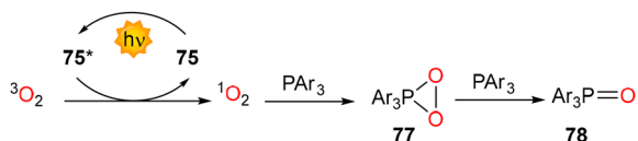
Fig. 18 Synthesis of phosphine oxide through aerobic oxidation.
