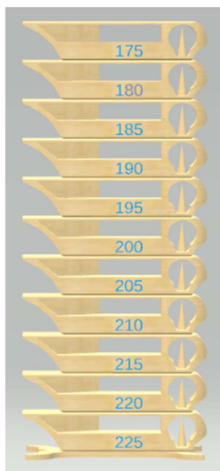
Fig. 1 Design photo of the calibration tower.
