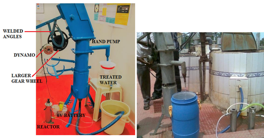
Fig. 11 Fitting of experimental setup on Pattikadu Oorani. The hand pump with gear wheel, shown on the left, was modified to drive a gear system linked to a dynamo, converting mechanical energy into electricity and charging a 6 V DC battery. The UV LED reactor is the silver cylinder in the bottom right of the right photo.
