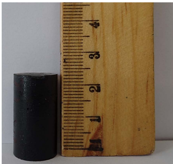
Fig. 3 Specimen used for the compressive strength test.
