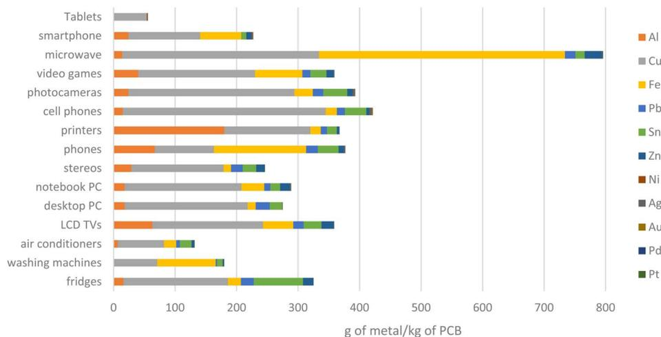
Fig. 3 Average metal composition in the most common electronic circuit boards.<sup>53–55</sup>
