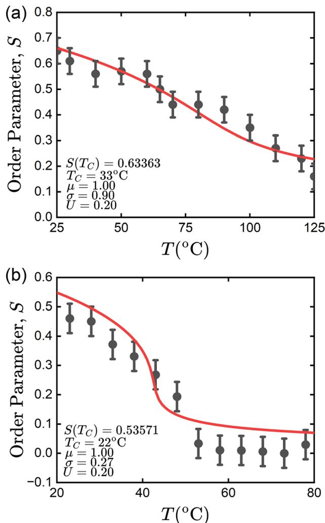
Fig. 4 Order parameter ( $S = \langle P_2 \rangle$ ) data obtained from Raman spectroscopy measurements for (a)  $1\times$  sample and (b)  $1/8\times$  sample. The red lines show the numerical fit to the data by solving eqn (16), with the relevant fitting parameters shown for each case.
