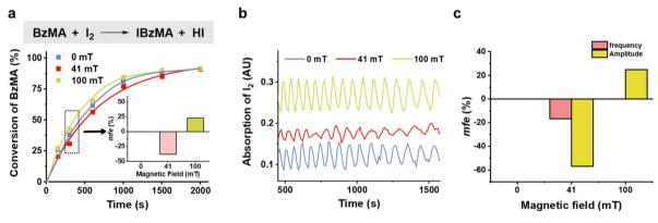
Fig. 2 MFEs on the conversion of BzMA. (a) Time trace of the BzMA conversion measured by HPLC at 0 mT (blue line), 41 mT (red line), and 100 mT (green line). (b) Time trace of  $I_2$  absorbance (460 nm) in BzMA oscillating systems at 0, 41, and 100 mT. (c) Comparison of *mfe* between frequency and amplitude in Fig. 2b.
