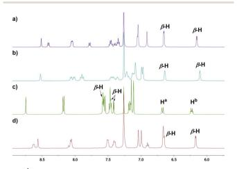
Fig. 2  $^{1}$ H NMR spectra of (a) **6** in CDCl<sub>3</sub> at 293 K; (b) **8** in CDCl<sub>3</sub> at 293 K; (c) **9** in CDCl<sub>3</sub> at 293 K; (d) **11** in CDCl<sub>3</sub> at 293 K.
