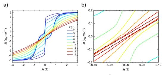
Fig. 3 (a) Hysteresis loops of 1-Dy from 2 to 16 K and -3 T to +3 T, sweep rate is 22 Oe s<sup>-1</sup>. (b) Hysteresis loops of 1-Dy at 6-16 K between -3 and +3 T zoomed in between -0.1 and +0.1 T, sweep rate is 22 Oe s<sup>-1</sup>. Hysteresis is considered open until  $T_{\rm H} = 14$  K.
