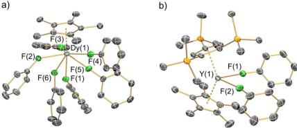
Fig. 2 Single crystal XRD structures of (a) the dication of 1-Dy and (b) the cation of 4-Y with selected atom labelling (Y/Dy: cyan, C: grey, F: green, Si: orange). Displacement ellipsoids set at 20% probability levels; hydrogen atoms, the lattice solvents and the counteranions have been omitted for clarity. See ESI† for selected bond lengths and angles.
