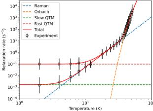
Fig. 4 Fitting of 1-Dy relaxation profile, showing Orbach, Raman and QTM components derived from egn (S5).† Error bars represent one ESD in the distribution of rates.
