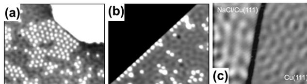
**Fig. 9** (a) and (b) STM images of Cu islands on the Cu(111) surface and Cu atoms at the edge, trapped by surface-mediated interaction, respectively. The mean Cu–Cu separation is approx. 12.5 Å. Interference patterns from FOs of different atoms may be visible. (c)  $dI/dV$  STM image of bilayer NaCl on Cu(111) and Cu(111). Panels (a)–(c) are reprinted with permission from the works of Repp *et al.*<sup>64</sup> as well as Repp and Meyer.<sup>82</sup>
