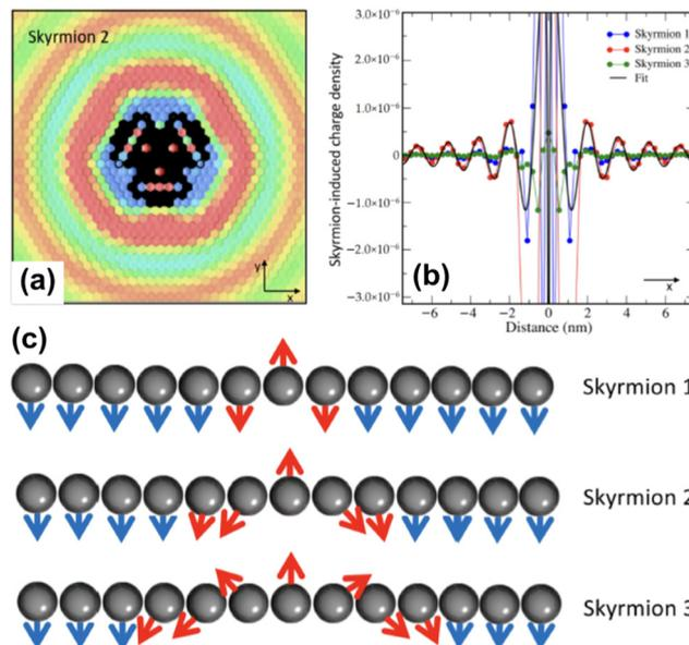
**Fig. 14** Skyrmion-induced charge oscillations in PdFe/Ir(111). (a) Ring-like ripples surrounding Skyrmion 2 at 2.15 eV. Atop the skyrmion, the charge is extremely large and thus removed to observe the surrounding oscillations. (b) Comparison of the Friedel oscillations along the  $x$ -direction as a function of the size of the confined noncollinear spin-textures shown side-wise in panel (c). Reprinted with permission from the work of Bouhassoune *et al.*<sup>108</sup>
