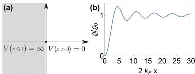
Fig. 6 (a) Plot of the hard-barrier surface introduced at  $x = 0$  and (b) plot of the resultant Friedel oscillations of charge density.<sup>15</sup>
