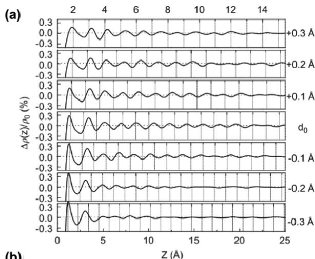
**Fig. 29** (a) FOs within the surface-truncated Al(110) bulk for various interlayer distances  $d_0$  along the ref. 108 direction, taken in steps of 0.1 Å. The  $z$  axis denotes the distance from the surface to the bulk, and the top abscissa depicts the index of the atomic layers. Reprinted with permission from the work of Li *et al.*<sup>153</sup> Panel (b) depicts a mathematical model of the surface of a crystal or a half-infinite space.<sup>16</sup>
