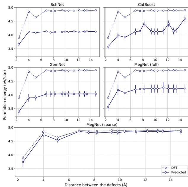
Fig. 31 The dependency of formation energies on the distance between defects in MoS<sub>2</sub> with one Mo and one S vacancy obtained with neural network approaches (SchNet, CatBoost, GemNet, MagNet) and DFT. Reprinted with permission from the work of Kazeev *et al.*<sup>155</sup>
