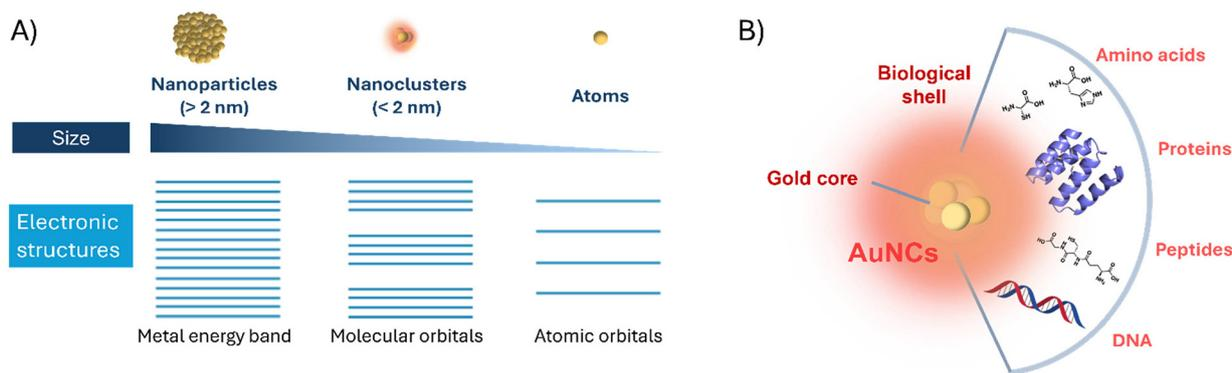
**Fig. 1** (A) Size-dependent electronic structure of metal nanomaterials showing gold nanoparticles with continuous electronic bands and gold nanoclusters with discrete energy bands. (B) Different biological molecules, such as amino acids, peptides, proteins or DNA, used as protecting agents in the synthesis of metal nanoclusters.
