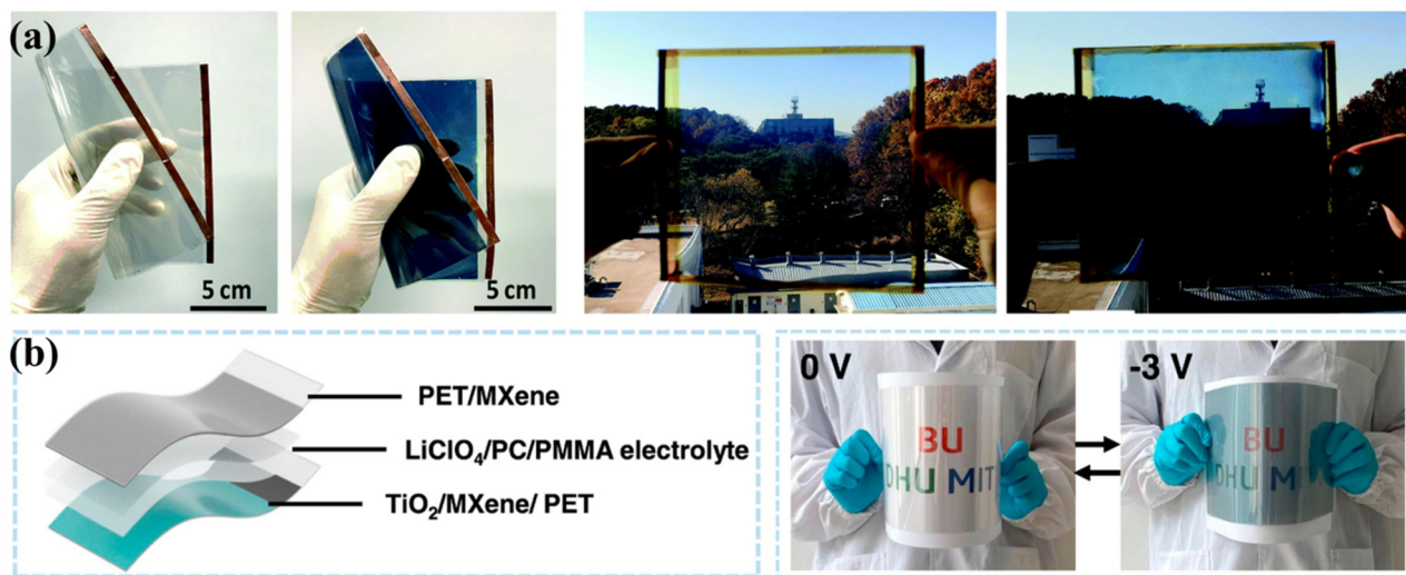
Fig. 8 (a) Photograph images of a flexible EC smart window. Reproduced with permission. 150 Copyright 2021 Royal Society of Chemistry. (b) Schematic diagram and large-area applications (about 20 × 30 cm) of the flexible solid ECD. Reproduced with permission. 151 Copyright 2021 Springer Nature.
