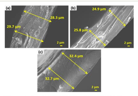
Fig. 7 Cross-sectional FESEM images of the (a) pure GG, (b) 5% PEDOT:PSS/GG, and (c) 20% PEDOT:PSS/PdPt/GG composite membranes.
