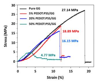
Fig. 9 Stress-strain PEDOT:PSS/GG curves composite membranes.
