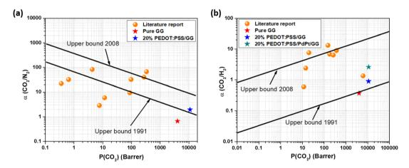
Fig. 11 Comparative assessment of gas separation performance against the Robeson upper bound and previously published work for (a) CO<sub>2</sub>/N<sub>2</sub> and (b) CO<sub>2</sub>/H<sub>2</sub> separation.
