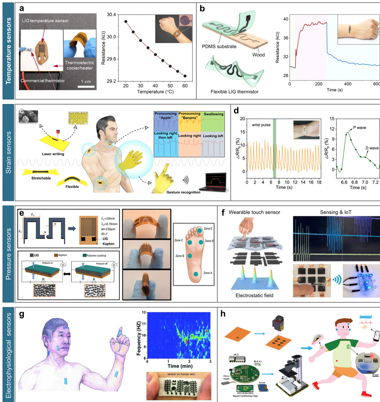
Fig. 7 (a) Left: Photograph of a LIG temperature sensor fabricated on a leaf and the experimental setup for performance evaluation. Right: Resistance–temperature response of the sensor over the range of 20–60 °C. Reproduced with permission. 9 Copyright 2019, Wiley-VCH Verlag. (b) Left: Transfer process of LIG from wood to a PDMS substrate. Right: LIG/PDMS temperature sensor used for monitoring human body temperature. Reproduced with permission. 63 Copyright 2021, Elsevier. (c) Application of a LIG-based strain sensor for tracking muscle movements and human motions. Reproduced with permission. 103 Copyright 2022, Springer Nature. (d) Left: Real-time signal captured by the F-LIG/PDMS sensor for wrist pulse monitoring. Right: Enlarged view of the shaded region showing distinct P-wave and D-wave components. Reproduced with permission. 75 Copyright 2024, Springer Nature. (e) Left: Schematic design and working principle of LIG-based pressure sensors. Middle: Photographs demonstrating the sensor's mechanical flexibility. Right: Placement of LIG pressure sensors on the foot for dynamic pressure mapping. Reproduced with permission. 20 Copyright 2020, John Wiley & Sons, Inc. (f) A triboelectric touch sensor comprising a 3 × 3 LIG electrode array, capable of wirelessly controlling LEDs. Reproduced with permission. 18 Copyright 2024, American Chemical Society. (g) Left: Schematic illustration of sensor placement on various body parts (forehead, chest, forearm, face, neck, and finger) for monitoring electrophysiological signals such as EEG, ECG, and EMG. Top right: Recorded alpha rhythm signal from the forehead. Bottom right: Photograph of the sensor. Reproduced with permission. 21 Copyright 2018, Wiley-VCH Verlag. (h) Fabrication process, concept, and photograph of a three-in-one portable electronic platform designed for simultaneous measurement of EEG, ECG, and EMG signals. Reproduced with permission. 116 Copyright 2023, Wiley-VCH Verlag.
