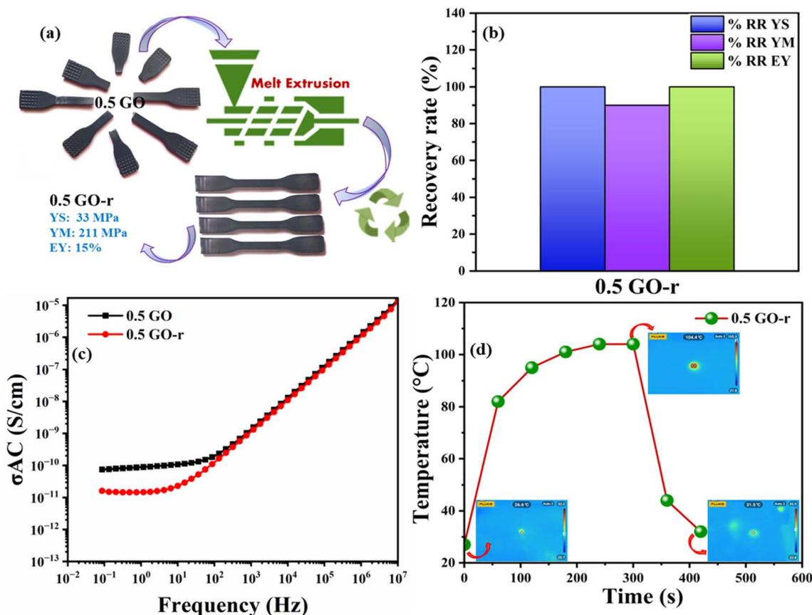
Fig. 8 Recyclability study of the PCR PP vitrimer nanocomposite. (a) Recycling scheme, (b) recovery rate of mechanical characteristics, (c) AC conductivity, and (d) temperature vs. time graph upon heating and cooling along with infrared thermal imaging for the vitrimer nanocomposite (0.5 GO-r) post recycling.
