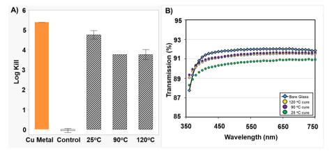
Fig. 7 Antimicrobial efficacy and optical transmission results for Ferro 221 glass coatings dosed with copper glass-ceramic (CGC) powder extracts with triethyl phosphite (TEP) ([Cu]<sub>Tot</sub> = 600 ppm) and cured at different temperatures. A. Average log-kill values against S. aureus for various coating cure conditions. Control sample has no antimicrobial additive. Error bars represent the standard deviation of duplicate samples. B. Optical transmission measurements.
