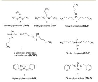
Fig. 2 Molecular structures of phosphite and phosphate chemicals tested in extractions from copper glass-ceramic powder.
