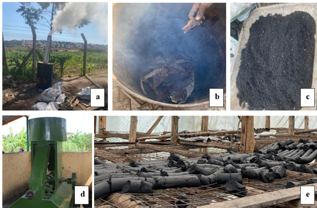
Fig. 1 (a) A metallic drum carbonisation kiln in use; (b) the carbonisation initiation with wood as a start-up fuel; (c) the produced faecal sludge char (ground); (d) the briquette extruder machine; and (e) the produced briquettes on drying racks (Lubigi Wastewater Treatment Plant, Kampala, Uganda).
