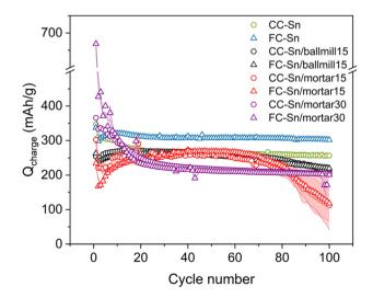
Fig. 7 Electrochemical performance of spray dried samples vs. composites made by other methods (hand ground and ball milled). Here we report samples prepared with 30 and 15 Sn wt% in a mortar and the samples prepared with 15 Sn wt% in ball milling jars.
