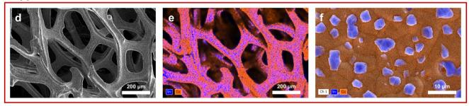
Fig. 2 SEM characterizations on Sn-deposited substrates after charging at 1 mA cm<sup>-2</sup> and 2 mAh cm<sup>-2</sup> in CEM-separated cells with 1.7 M Sn electrolyte. (a-c) Graphite felt substrate. (a) Overview. (b) EDS mapping of (a). (c) Zoom-in EDS mapping. (d-f) Cu foam substrate. (d) Overview. (e) EDS mapping of (d). (e) Zoom-in EDS mapping. EDS mapping are false-colored images where the colors represent elemental distributions: blue for Sn, red for C, and orange for Cu.
