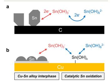
Scheme 1 Schematic representation of the bi-directional promoter effect of Cu in the four-electron Sn(OH)<sub>6</sub><sup>2-</sup>/Sn redox system. (a) On a C-based substrate. (b) On a Cu-based substrate.
