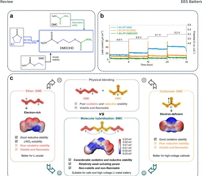
Fig. 2 (a) Design rationale of DMDOHD. (b) Potentiostatic floating profiles of Li|LNMO cells with various carbonate-based electrolytes. Reproduced with permission.<sup>34</sup> Copyright 2024, Springer Nature. (c) Schematic illustration of BMC molecule design. Reproduced with permission.<sup>35</sup> Copyright 2024, Springer Nature.
