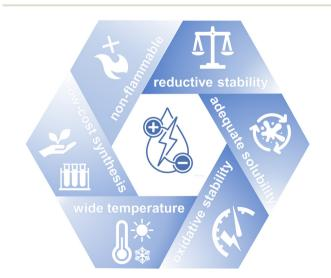
Fig. 1 Illustration of the design criteria for the solvent molecule in LMB electrolytes.
