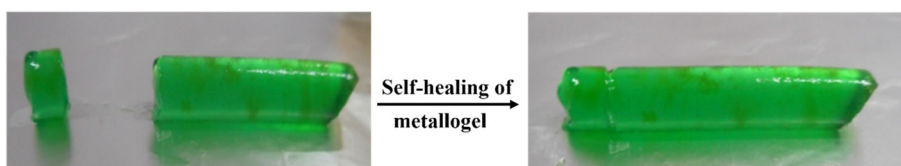
Fig. 8 Demonstration of the self-healing property of MG1 (prepared using 12 mM \text{Cu}^{2+} salt with 1 : 1 \text{Cu(II)} : gelator in methanol).
