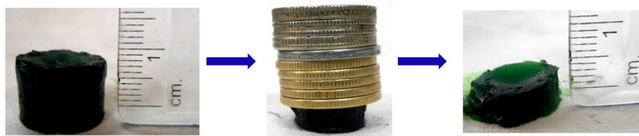
Fig. 7 Demonstration of the self-sustaining property of a metallogel (prepared using 6 mM \text{Cu}^{2+} salt with 1 : 1 \text{Cu(II)} : gelator in methanol). The weight of each Indian currency coin is 5 g.
