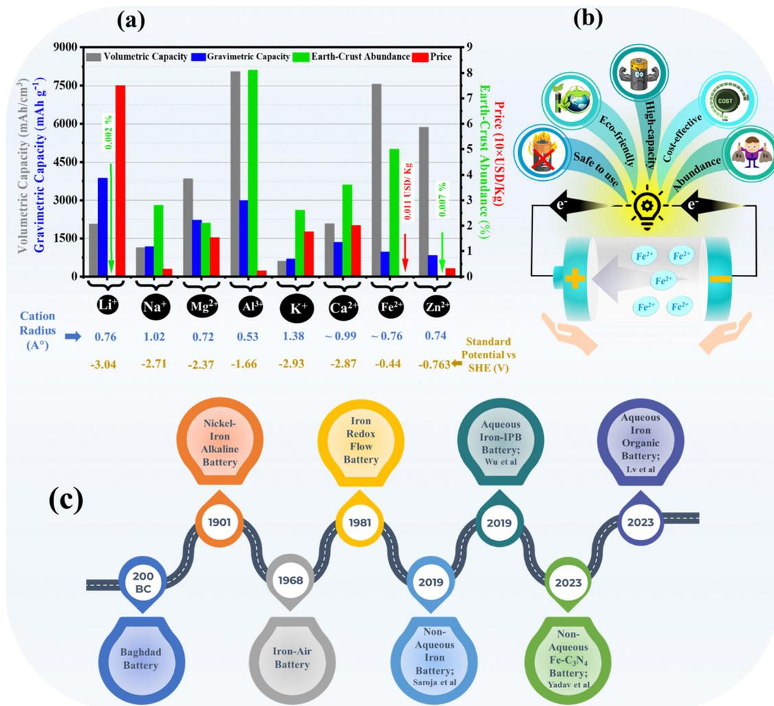
**Fig. 1** (a) Various mono and multivalent metal-ion battery parameters in terms of volumetric capacity, gravimetric capacity, earth-crust abundance percentage, price, cation radius, and standard potential vs. SHE. (b) Schematic representation of the characteristics of Fe-ion batteries. (c) Timeline of the progress in iron metal-based rechargeable batteries.
