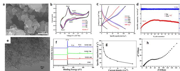
Fig. 7 (a) SEM image of DADB. (b) CV curve of DADB under  $0.2 \text{ mV s}^{-1}$ . (c) GCD of DADB under  $0.05 \text{ A g}^{-1}$ . (d) Cyclic stability of DADB under  $1 \text{ A g}^{-1}$ . (e) HRTEM images of TOMC-700. (f) XPS survey of the sample. (g) Specific capacitance at a series of current densities. (h) EIS spectrum of the ZHSC cathode respectively.
