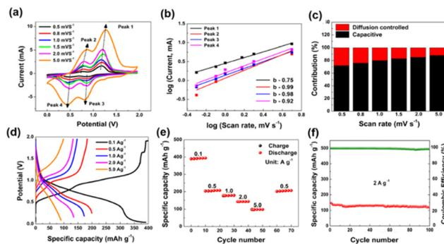
**Fig. 2** (a) CV curve at different scan rates. (b) Four primary redox CV peaks in a fitted plot. (c) Diffusion control and capacitive ratios at various scan rates. (d) GCD curves at different current densities. (e) Rate performance and (f) cyclic stability and coulombic efficiency @  $2 \text{ A g}^{-1}$  for the  $\text{V}_6\text{O}_{13}$  cathode respectively.<sup>8</sup>
