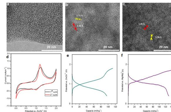
**Fig. 4** (a) STEM image of amorphous ( $\text{FePO}_4$ ). (b) Chemically sodiated. (c) Lattices fringe widths of lithiated ( $\text{FePO}_4$ ). (d) CV of amorphous ( $\text{FePO}_4$ ) versus zinc. (e) Electrochemical study of zinc insertion of amorphous ( $\text{FePO}_4$ ). (f) Electrochemical study of magnesium cell insertion of amorphous ( $\text{FePO}_4$ ).
