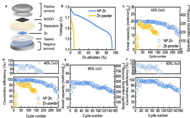
**Fig. 3** (a) Schematic of Zn || NiOOH coin cell. (b) Various anodes for zinc are used in primary Zn || NiOOH alkaline anodes. (c) Cycle number vs. discharging capacities of NP Zn and Zn powder sample. (d) Coulombic efficiency of NP Zn and Zn powder at 40% DoD. (e) At 60% depth of DoD, discharging capacities of the NP Zn anodes. (f) Coulombic efficiency of the sample at 60% DoD.
