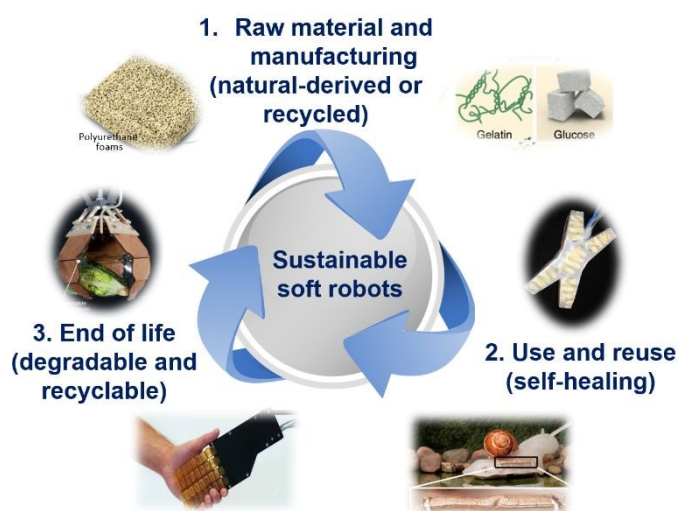
Fig. 1 The life cycle assessment of sustainable soft robots. Three main phases are classified from cradle to grave. Raw materials that are natural or recycled and manufacturing encode the original sustainable character at the start-of-life. Self-healing enables to reuse and refunction from damage at the middle-of-life. Degradable and recyclable allows degradation and recycle into a new life at the end-of-life instead of being discarded directly. Reproduced from ref. 59; Copyright 2023, Springer Nature. Reproduced from ref. 60; Copyright 2020, Springer Nature. Reproduced from ref. 38; Copyright 2022, the American Association for the Advancement of Science. Reproduced from ref. 34; Copyright 2023, Springer Nature. Reproduced from ref. 63; Copyright 2023, the American Association for the Advancement of Science. Reproduced from ref. 65; Copyright 2017, the American Association for the Advancement of Science.
