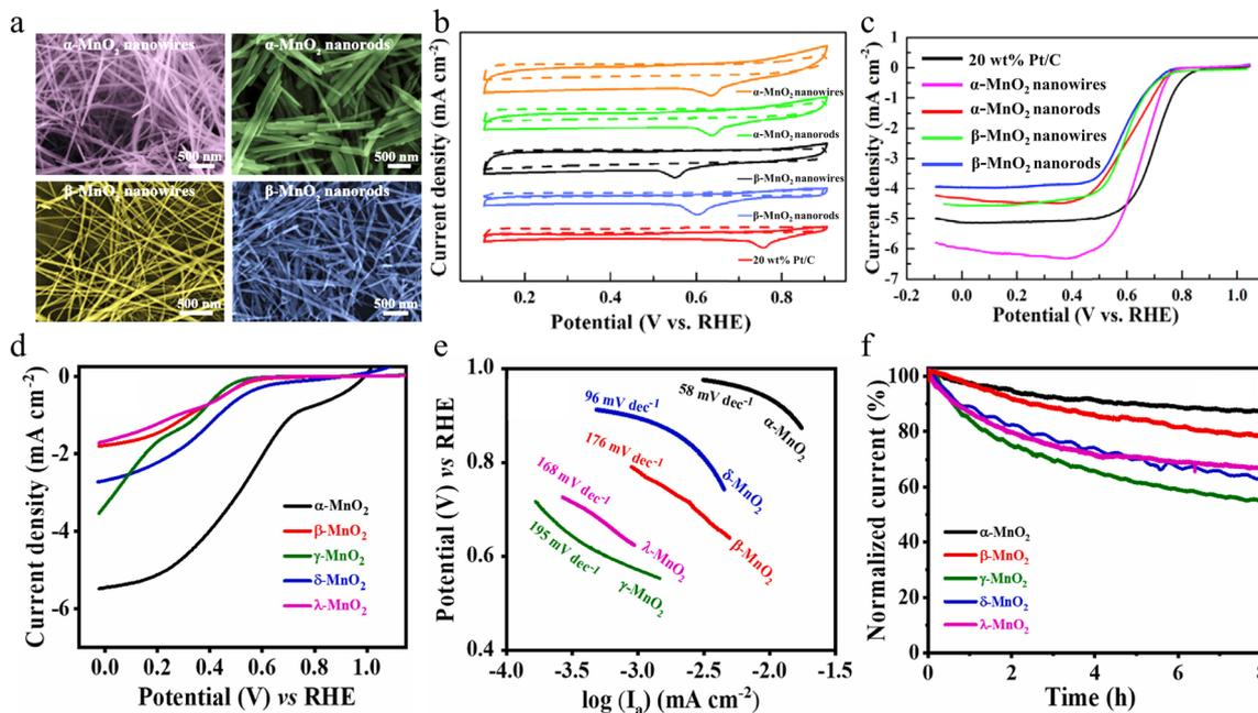
Fig. 3 The ORR performance and surface morphology of different  $\text{MnO}_2$ . (a) SEM images of the samples obtained. (b) CV curves and (c) LSV curves of the obtained  $\text{MnO}_2$  and 20 wt% Pt/C. Reproduced with permission.<sup>59</sup> Copyright 2019, Elsevier. (d) LSV curves, (e) Tafel slope and (f) chronoamperograms of  $\text{MnO}_2$  with different crystal structures. Reproduced with permission.<sup>60</sup> Copyright 2023, Elsevier.
