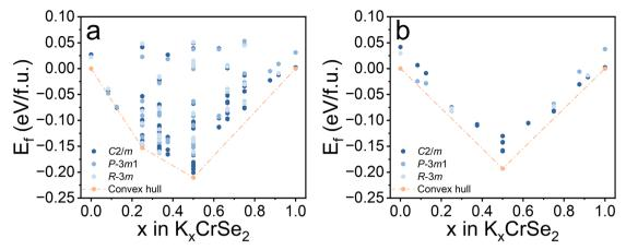
Fig. 4 Formation energies  $E_f$  of the one-dimensional phase space  $K_x CrSe_2$  ( $0 \le x \le 1$ ) evaluated with (a) the PBE functional and (b) the SCAN functional. The compounds on the convex hull of stability are highlighted in red.
