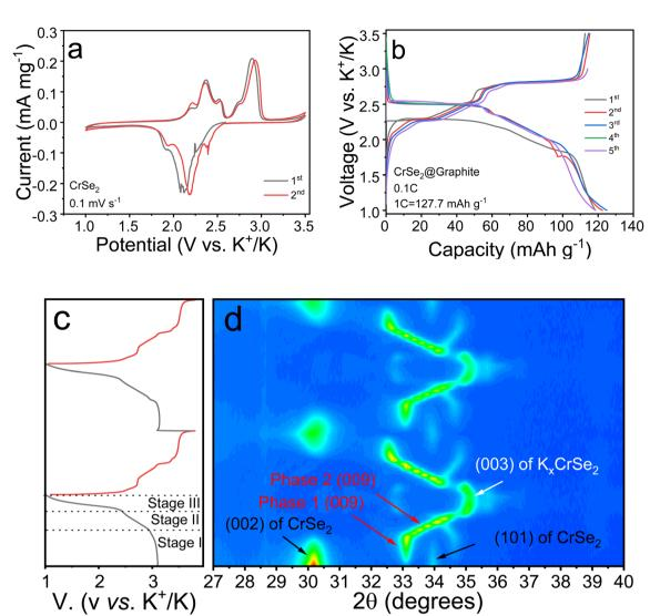
Fig. 3 (a) CV profiles of CrSe<sub>2</sub> recorded at 0.1 mV s<sup>-1</sup>, (b) GCD profiles of CrSe<sub>2</sub> recorded at 0.1C scan rate at 20 °C  $\pm$  2 °C. (c) GCD profiles of CrSe<sub>2</sub> and (d) corresponding contour plot of in operando PXRD data. The Miller indexes of key reflections of the expected phases are provided within the figure.
