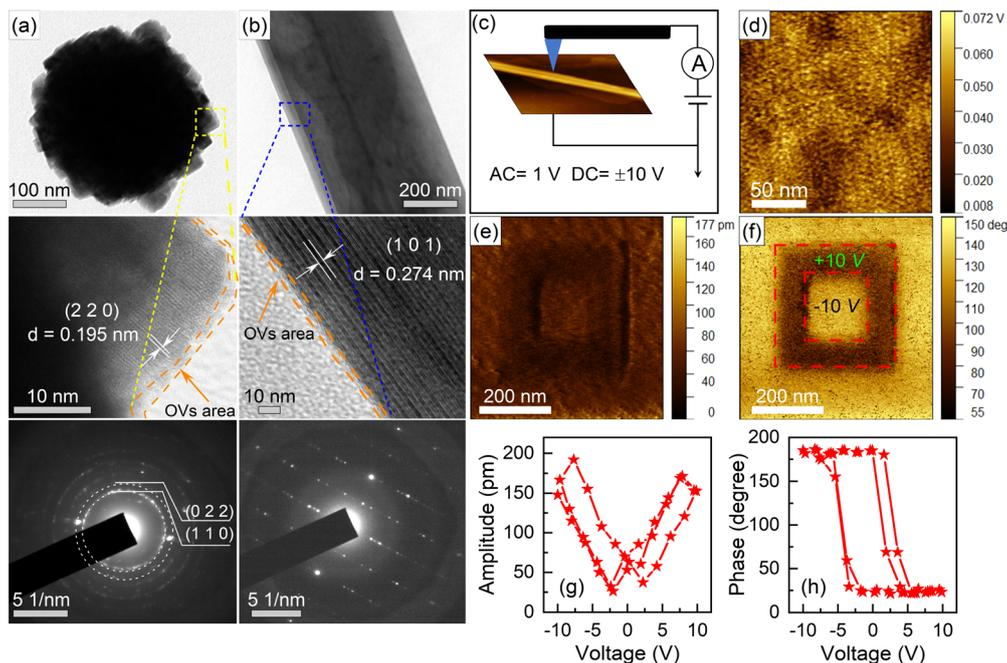
Fig. 2 (a and b) Micromorphology, local HR-TEM images and the corresponding electron diffraction patterns of nanospheres and nanobelts, respectively, for BNT- $V_{\text{O}}$ . (c) Schematic for PFM measurement of a nanobelt on a Ag/Si substrate. (d) KPFM potential images. (e) PFM amplitude and (f) phase scans of BNT with a box-in-box pattern obtained by the applications of reverse dc biases. (g) Amplitude butterfly and (h) phase hysteresis loops versus voltage.
