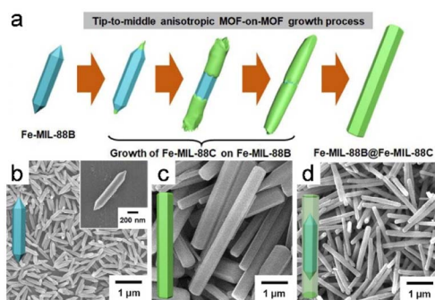
Fig. 4 (a) Schematic diagram of the apical to intermediate anisotropic MOF-on-MOF growth process. SEM images of (b) initial hexagonal rods of Fe-MIL-88B template, (c) pure Fe-MIL-88C hexagonal rods, and (d) Fe-MIL-88B@Fe-MIL-88C core–shell hybrid hexagonal rods. (Panels a–d) Reproduced with permission. 18 Copyright 2020, American Chemical Society.
