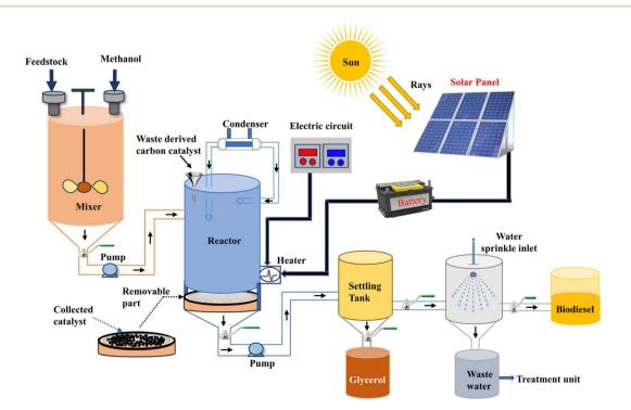
Fig. 14 Proposed reactor design for biodiesel production employing heterogeneous catalytic transesterification.
