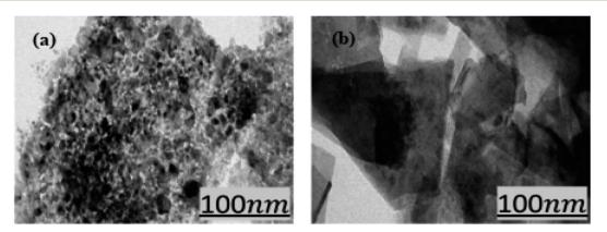
Fig. 7 TEM of the zeolite (a) and composite (b). Reprinted with permission from ref. 146. Copyright (2021) Elsevier.
