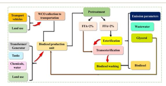
Fig. 13 The system boundary of a second-generation biodiesel production system. Reprinted with permission from ref. 375. Copyright (2020) Elsevier. \*FFA – free fatty acid.
