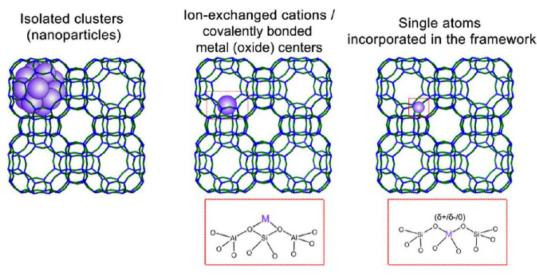
Fig. 6 Possible zeolite-metal composite configurations. Reprinted with permission from ref. 285. Copyright (2018) ACS.
