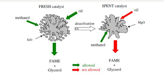
Fig. 8 Scheme for the catalyst deactivation process. Reprinted with permission from ref. 308. Copyright (2012) Elsevier.
