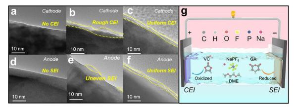
Fig. 6 The mechanism analysis of electrolytes. HRTEM images of NVP in (a) 1 M NaPF $_6$  + DME, (b) 1 M NaPF $_6$  + DME/VC and (c) 1 M NaPF $_6$  + DME/VC + 2 wt% GA electrolytes. HRTEM images of HC in (d) 1 M NaPF $_6$  + DME, (e) 1 M NaPF $_6$  + DME/VC and (f) 1 M NaPF $_6$  + DME/VC + 2 wt% GA electrolytes. (g) The illustration of film formation on the cathode and anode in 1 M NaPF $_6$  + DME/VC + 2 wt% GA electrolytes.
