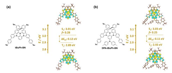
Fig. 3 Difference density plots and energies of  $S_1$  and  $T_1$  calculated in the gas phase at SCS-(ADC)2/cc-pVDZ level, respectively, for (a) tBuPh-BN and (b) DPA-tBuPh-BN (Blue indicates an area of decreased electron density while yellow indicates increased electronic density between the ground and excited states).
