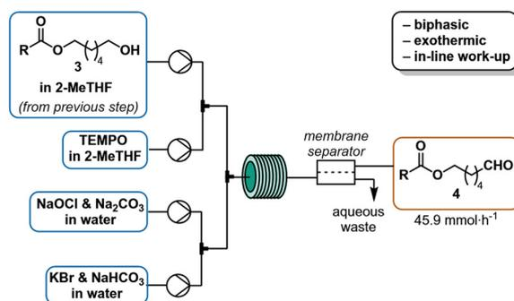
**Scheme 4** Oxidation of primary alcohol **3** to aldehyde **4**. Reaction conditions: ester **3** in 2-MeTHF (0.72 M, 1 equiv., from previous step), TEMPO in 2-MeTHF (7 mol%, 0.5 M), 2.3 equiv. aqueous hypochlorite (NaOCl, 2 M and Na<sub>2</sub>CO<sub>3</sub>, 0.3 M in water) and 0.35 equiv. aqueous potassium bromide (KBr, 0.25 M and NaHCO<sub>3</sub>, 0.7 M in water) are reacted at room temperature for 2.3 min.
