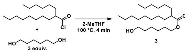
A solution of 1,6-hexanediol in 2-MeTHF (2.50 M) was delivered by a HPLC pump (1.5 mL min<sup>-1</sup>) and combined with the acid chloride stream *via* a T-mixer. The resulting stream was heated at 100 °C for 4 min (10 mL reactor). Aqueous sodium hydroxide (1 M) was pumped by an HPLC pump (5.5 mL min<sup>-1</sup>) and joined with the acylation stream *via* a T-mixer. The resulting flow was cooled at 0 °C with a residence time of 1.25 min (10
