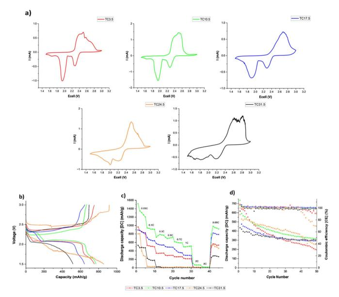
Fig. 5 (a) Cyclic voltammograms at 0.05 mV s<sup>-1</sup> scan rate before cycling; (b) initial charge discharge profiles at 0.5C; (c) discharge capacity during rate capability testing; (d) discharge capacity and coulombic efficiency at 0.1C during 50 cycles. All tests were performed for all TC cathodes in coin cell configurations at room temperature.
