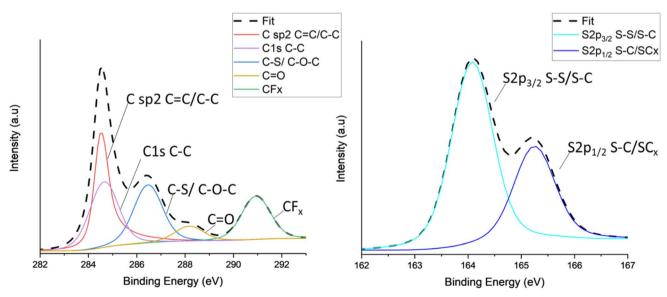
Fig. 4 XPS peaks for TC10.5 with (a) C 1s; (b) high resolution S 2p spectra.
