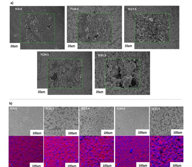
Fig. 2 (a) SEM images of the magnified surface morphology of different types of cathodes; (b) overview SEM images and the corresponding EDX elemental mapping of the cathode surface morphology. Fig. S1 in ESI† shows SEM images of TC10.5 cathode film and vs. TC10.5 composite powder. Table ST1 in ESI† shows EDX mass and atomic% of all cathode samples.
