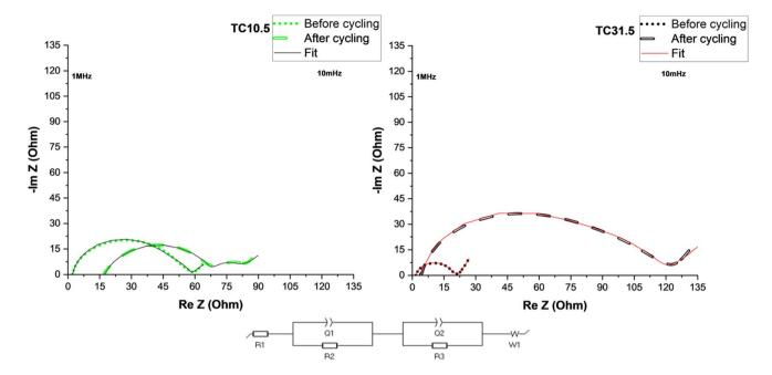
Fig. 6 EIS plots of TC10.5 and 31.5 before and after 50 cycles at 0.1C.
