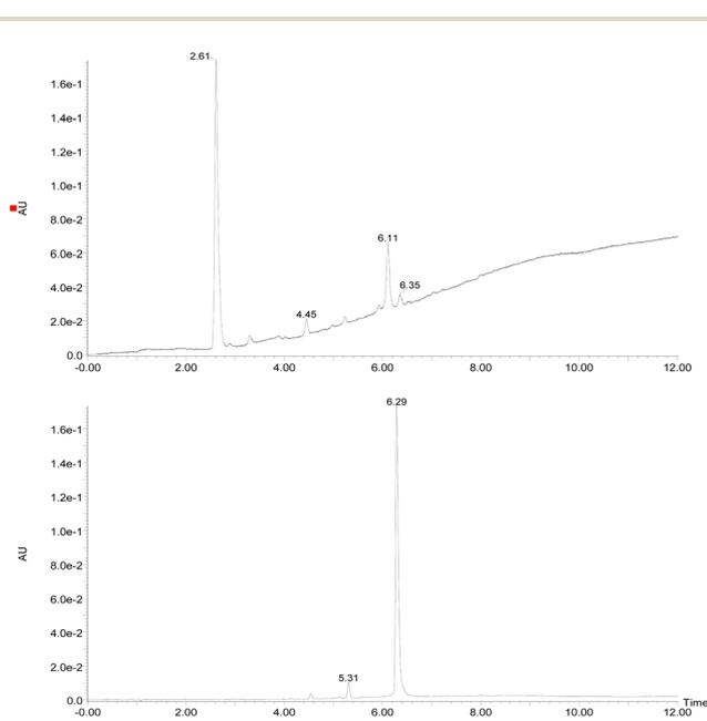
Fig. 2 Chromatogram DAD (240–700 nm) (top of the image) obtained from the crude extract of the *Cordyceps* sp. and (bottom of the image) obtained after dehydration reaction of the crude extract. (RT = 2.61 min (erythrostrominone) and RT = 6.29 min (3,5,8-TMON)).
