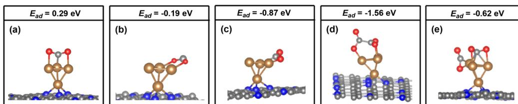
Fig. 2 The key geometric parameters and adsorption energy analysis of the possible adsorption configuration of the CO<sub>2</sub> molecule on the Cu<sub>4</sub>/N<sub>3</sub>GN catalyst with the (a) top, (b) bridge\_1, (c) bridge\_2, (d) coupling and (e) isolating models.
