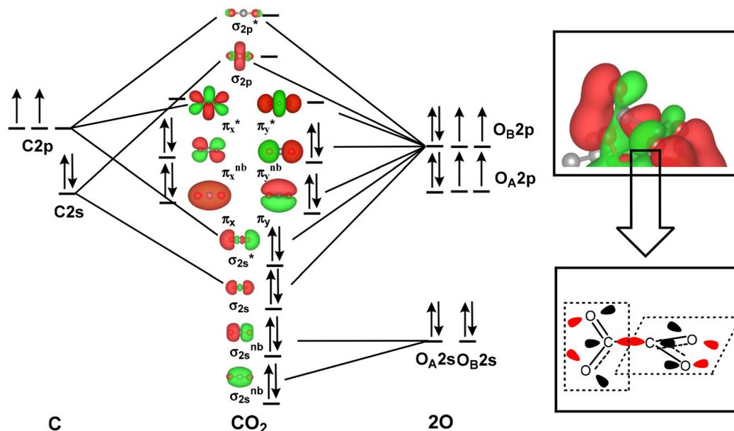
**Fig. 4** The frontier molecular orbitals of free carbon dioxide molecules and the HOMO of the  $^*\text{OOCO}^*\text{O}^*$  dimer, highlighting that the effective overlapping of two distorted  $\pi^*$  antibonding orbitals of two bent  $\text{CO}_2$  molecules results in the formation of the C–C bond in the  $\text{CO}_2$  dimer.
