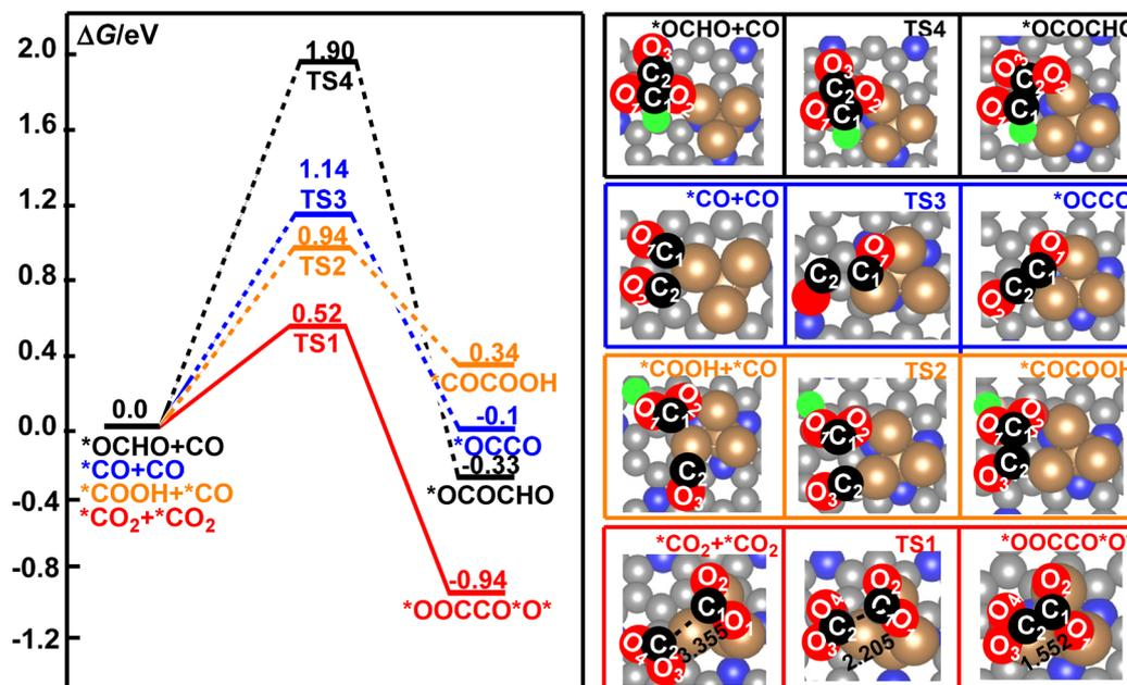
**Fig. 3** The calculated free energy profiles for the direct coupling of two  $^*CO_2$ ,  $^*OCHO$  and  $CO$ ,  $^*COOH$  and  $^*CO$ , and two  $CO$  molecules to form a C–C bond on the surface of the  $Cu_4/N_3GN$  catalyst.
