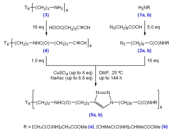
**Scheme 1** Triglycine/trialanine methyl ester (1a/b) N-terminus modification with 6-azido-hexanoic acid to produce 6-azido-hexanoyl-triglycine methyl ester (2a), and 6-azido-hexanoyl-trialanine methyl ester (2b). Subsequent CuAAC “clicking” of  $T_8[N\text{-propyl-hex-5-ynamide}]_8$  (4) and 6-azido-hexanoyl-triglycine/trialanine methyl ester (2a/b) to form  $T_8$ POSS-[triglycine/trialanine methyl ester]<sub>8</sub> (5a/b).
