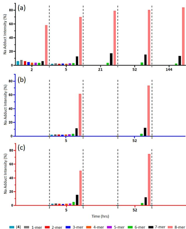
**Fig. 2** (a–c) MALDI-ToF mass spectra of multi-mer species  $[n\text{-mer} + \text{Na}]^+$  adduct intensities (relative percentages (%)) of timed “clicks” between (2a) and (4) using  $\text{CuSO}_4$  (4.0 eq.) and Na ascorbate (4.4 eq.) at different temperatures: 25 °C aliquots at 2-, 5-, 21-, 52- and 144-h (a), 15 °C aliquots at 5- and 52-h (b), and 35 °C aliquots at 5- and 52-h (c) (full spectra shown in ESI S40–S51†).
