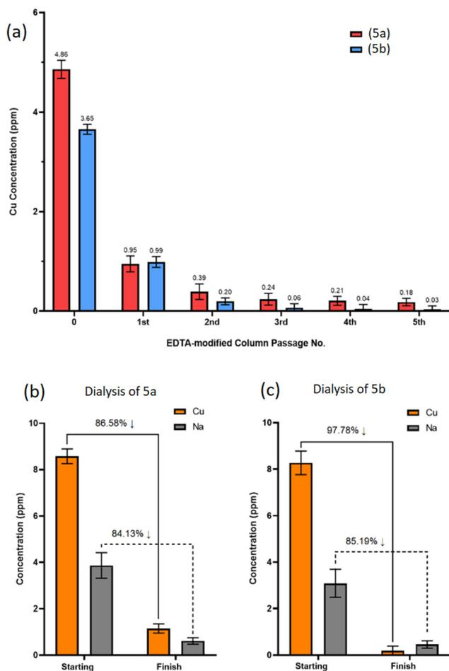
**Fig. 7** ICP-OES measurement of residual Cu concentration (ppm) in crude products (5a) and (5b), with subsequent Cu concentrations following passage through EDTA-modified Amberlite $\text{\textcircled{R}}$  columns (a). Starting Cu and Na concentrations, alongside final concentrations following 7  $\times$  dissolution media changes during dialysis for product (5a) (b) and product (5b) (c).
