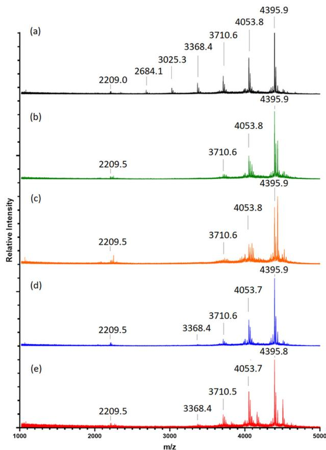
**Fig. 1** MALDI-TOF mass spectra at 72-h following “clicks” between (2a) with (4) in contrasting CuSO<sub>4</sub> equivalents listed in Table 1 (A–E) (a–e), respectively. Full spectra shown in ESI S35–S39.†
