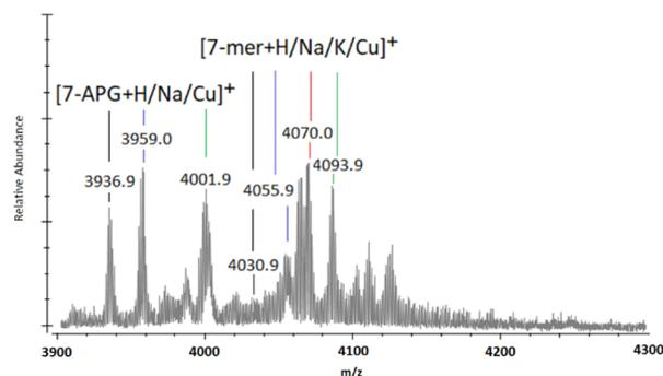
**Fig. 3** MALDI-ToF mass spectra between  $m/z$  3900 and 4300 showing multi-mer species following 72-h of “clicking” between (2a) and (4), using  $\text{CuSO}_4$  (4.0 eq.) and Na (4.4 eq.) (the full spectra of the example shown in this figure is presented in ESI S46†).
