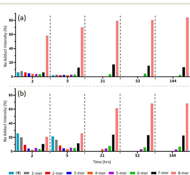
**Fig. 6** MALDI-TOF mass spectra of multi-mer species [*n*-mer + Na]<sup>+</sup> adduct intensities (relative percentages (%)) of timed “clicks” using 4.0 eq. CuSO<sub>4</sub> and 4.4 eq. Na ascorbate at 2, 5, 21, 52 and 144 h between (2a) and (4) (a) (full spectra shown in ESI S40–S47†), and between (2b) and (4) (b). (Full spectra shown in ESI S67–S71.†)
