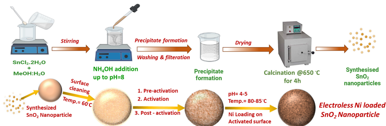
Fig. 1 Process schematic for the synthesis of SnO 2 nanoparticles and their electroless loading with Ni.
