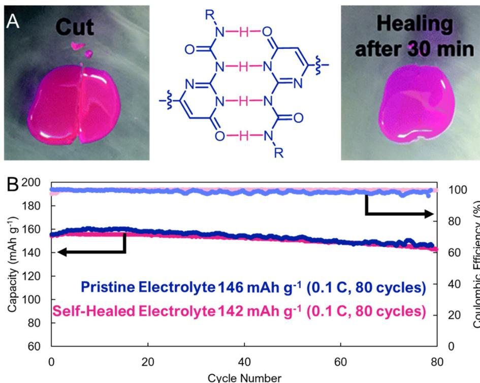
**Fig. 10** (A). Optical images showing the self-healing process of the ureidopyrimidinone-based electrolyte. (Left) The sample was cut into two pieces and (Right) after 30 minutes at 60 °C self-healing was observed. (B). Cycling stability comparing a cell containing pristine electrolyte, and electrolyte that has been cut, and then self-healed. Adapted with permissions from ref. 57. Copyright © 2018 Royal Society of Chemistry.
