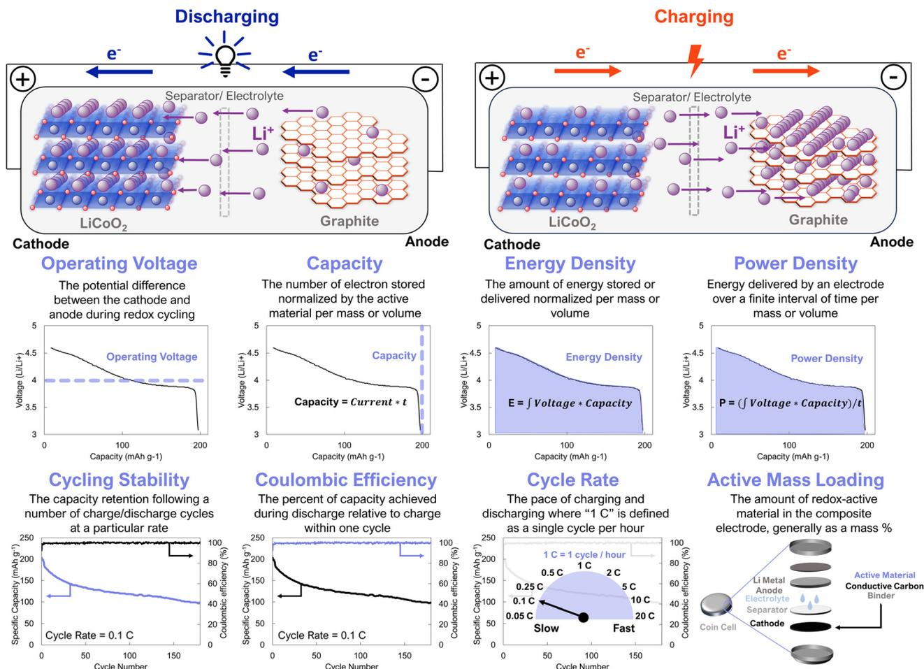
**Fig. 1** Schematic of battery charging/discharging processes and common performance metrics to evaluate new electrode active materials. Data is for  $\text{LiCoO}_2$ , which was adapted with permissions from ref. 5. Copyright © 2022 Wiley.
