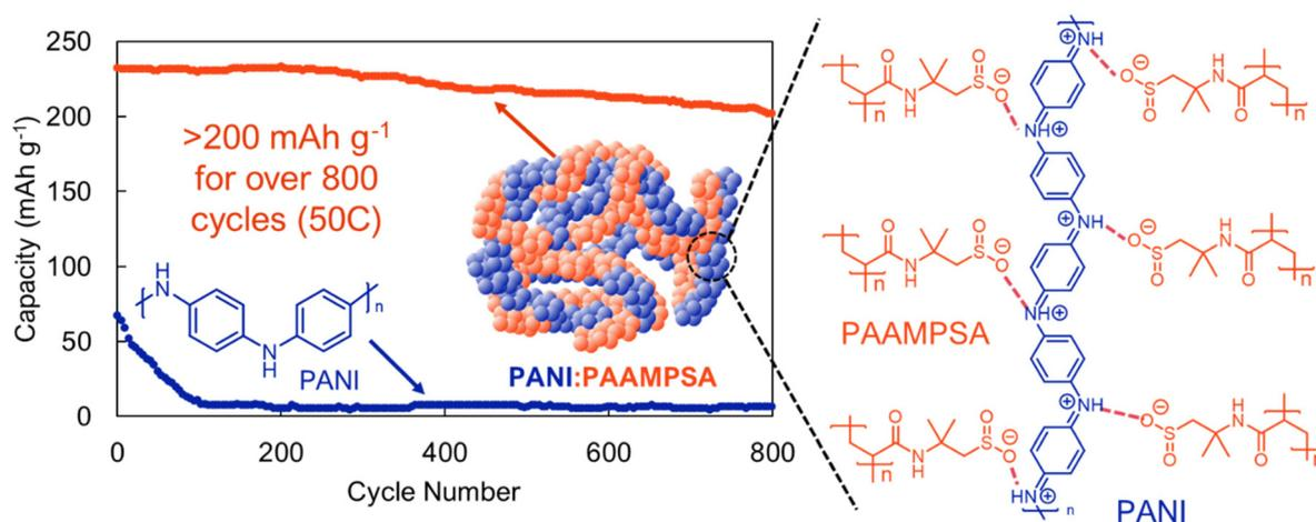
**Fig. 11** Cycling of a pernigraline-polyaniline with a polyacid stabilizer (PANI:PAAMPSA) (orange) compared to pure polyaniline (PANI) (blue) at a 50C rate. Adapted with permissions from ref. 57. Copyright © 2013 Royal Society of Chemistry.
