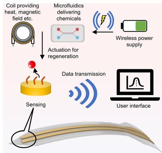
**Fig. 7** Schematic illustration of a proposed regenerable *in vivo* biosensor for real-time monitoring, as discussed in this mini-review. The integration of sensing and actuation elements will facilitate the dissociation of analytes from the device upon an external stimulus transmitted to the system wirelessly.
