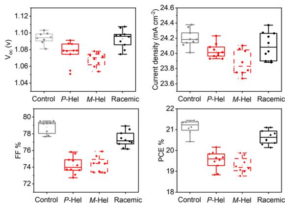
Fig. 3 Photovoltaic device performance. Photovoltaic metrics of control (black) and helically modulated (in color) devices. Representative  $J-V$  curves and photovoltaic performances for other perovskite compositions and preparation procedures are shown in the ESI (Experimental section and Fig. S25 and S26†).
