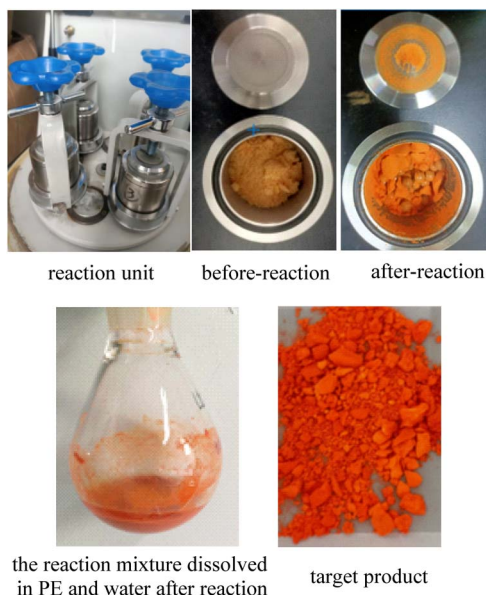
Fig. 1 Ball milling setup and process.
