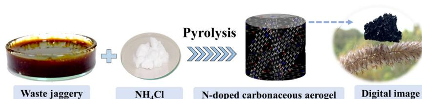
Scheme 1 Schematic of the synthesis of ultralight N-CA using waste jaggery and NH<sub>4</sub>Cl as precursors.
