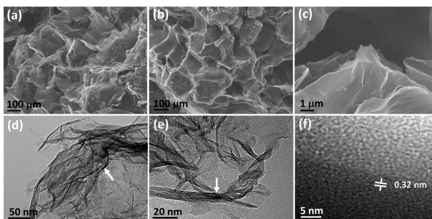
Fig. 1 (a–c) FE-SEM images of N-CA, (d and e) low-magnification TEM images (the white arrow indicates multilayer graphene) and (f) HR-TEM image of N-CA (the white line shows the inter layer distance).
