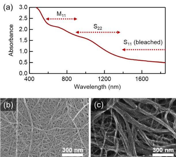
**Fig. 2** Aqueous dispersion of SWCNTs using amsonic acid, FB28, and FB220. (a) Absorption spectrum of SWCNTs in water in the presence of 0.1 wt% amsonic acid. Due to the optical window of solvents, the absorption spectrum is shown below 1800 nm. Scanning tunnelling electron microscopy (STEM) images of SWCNTs dispersed (b) with and (c) without 0.1 wt% amsonic acid aqueous solution.
