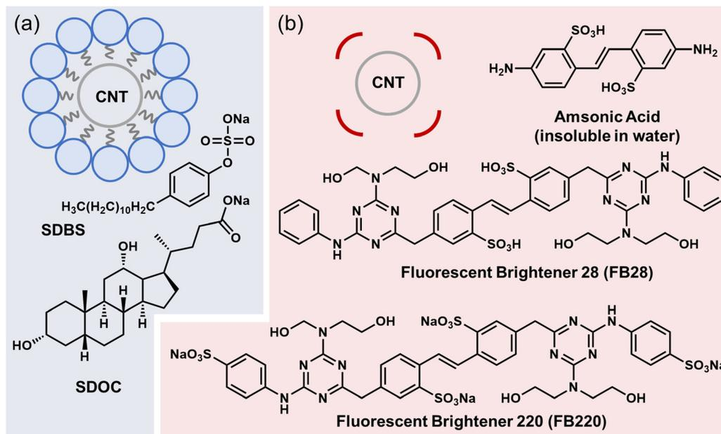
**Fig. 1** Surfactant structures. (a) Typical micelle-type surfactants. (b) Non-micellar surfactants. Abbreviations: CNT, carbon nanotube; SDBS, sodium dodecylbenzenesulfonate; SDOC, sodium deoxycholate.
