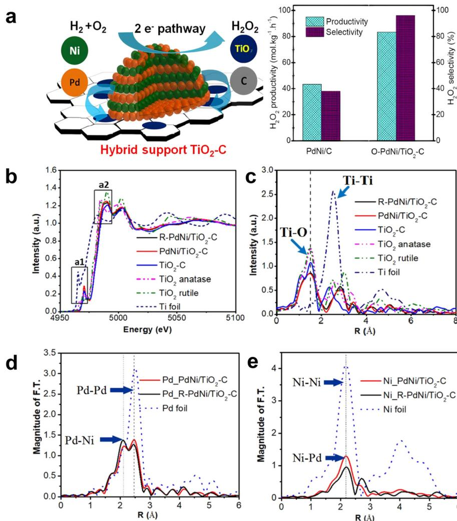
Fig. 6 (a) Schematic diagram of the reaction mechanism and performance comparison of the PdNi bimetallic catalyst supported by the C and TiO<sub>2</sub> mixed support. (b) XANES spectra of Ti K-edge and (c) EXAFS spectra of TiO<sub>2</sub>-C, PdNi/TiO<sub>2</sub>-C, and O-PdNi/TiO<sub>2</sub>-C. EXAFS spectra of (d) Pd and (e) Ni in PdNi/TiO<sub>2</sub>-C and R-PdNi/TiO<sub>2</sub>-C. <sup>36</sup> Copyright 2021, American Chemical Society.
