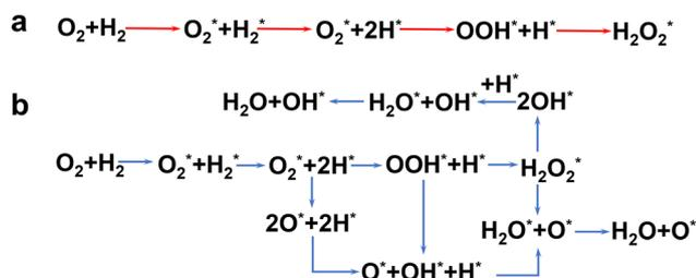
Fig. 3 Schematic diagram of the elementary reaction step network of the (a) main reaction and (b) side reaction for direct synthesis of  $\text{H}_2\text{O}_2$  from  $\text{H}_2$  and  $\text{O}_2$ .<sup>60</sup> Copyright 2017, American Chemical Society.
