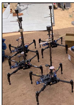
Fig. 9 Four instrumented multirotors used in the campaign.
