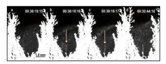
Fig. 10 Video frames from the same area, showing an ice needle formation by a non-classical crystallization<sup>69</sup> mechanism. There is no sign of a needle in frame (a) but it appears faintly in the following frame. Needle contrast and thickening increases from (b)-(d). The time difference between consecutive frames is 0.04 s.
