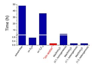
Fig. 12 Time to complete the reaction between quadricyclane and dimethyl azodicarboxylate in different solvents. Data from Sharpless 2005.<sup>84</sup>
