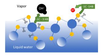
Fig. 5 Schematic representation of covalent and hydrogen bonds needed to release a hydronium ion or a hydroxide ion from a neutral water surface to the atmosphere, independent of the solvation of the ions. Releasing the positive ions requires less bond-breaking and thus lower energy than releasing hydroxide ions. C refers to a covalent bond and HB refers to a hydrogen bond.
