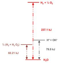
Fig. 13 Diagram showing the standard Gibbs energy levels for water, hydrogen peroxide, the ions formed by water self-ionization, and H2 +  $\frac{1}{2}$ O<sub>2</sub>. Reprinted with permission from ref. 131. Copyright 2023. American Chemical Society.
