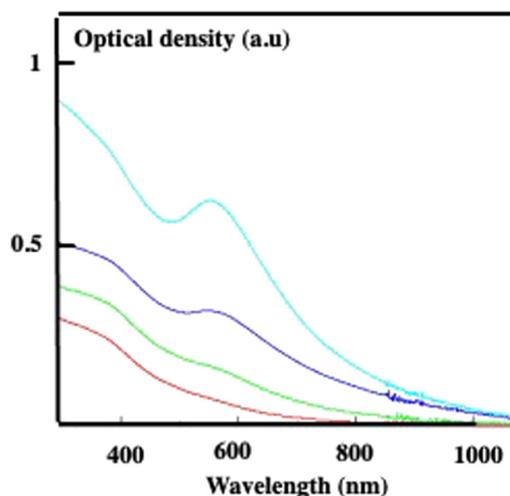
Fig. 10 Absorption of nano-eggs differing by their amount of Au nanocrystals involved in the aggregate. The percentage of Au compared to  $\text{Fe}_3\text{O}_4$  is (a) 10% red, (b) 60% green, (c) 100% blue and (d) 200% light blue.
