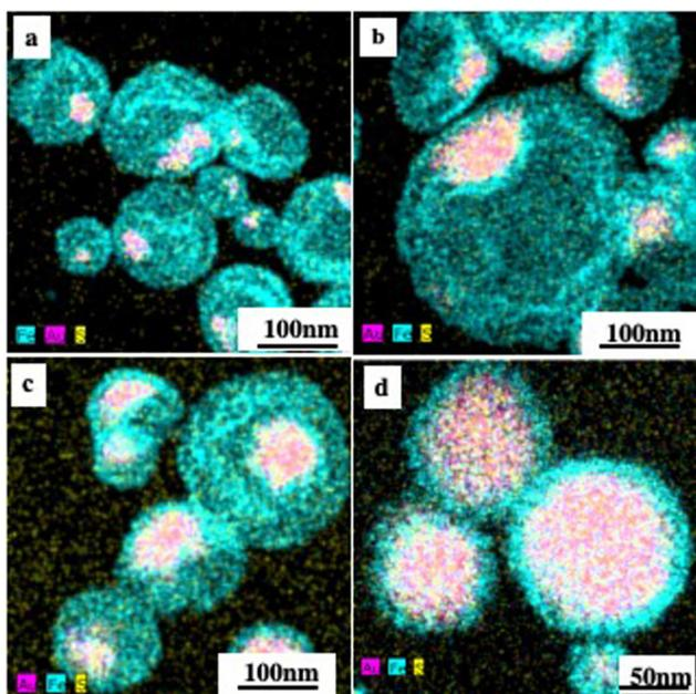
Fig. 7 EDS mapping (a)–(d) overview of “egg” superstructures of 10 nm  $\text{Fe}_3\text{O}_4$  nanocrystals ( $2 \text{ mg mL}^{-1}$ ) and 5 nm Au NCs differing by their amounts such as  $10 \text{ mg mL}^{-1}$  (a),  $60 \text{ mg mL}^{-1}$  (b),  $100 \text{ mg mL}^{-1}$  (c) and  $200 \text{ mg mL}^{-1}$  (d). Cyan, magenta and yellow denote Fe, Au and S elements respectively.
