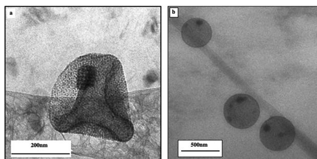
Fig. 8 Cryo-TEM image of a single colloidosome assembled from the  $\text{Fe}_3\text{O}_4/\text{Au}$  binary mixture.<sup>20</sup>
