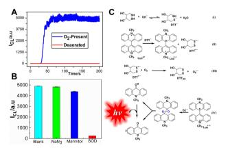
Fig. 6 (A) The effect of dissolved oxygen on the DTT/lucigenin system. Flow rate: 1.5 mL min<sup>-1</sup>; [lucigenin]: 10 μM; [DTT]: 0.3 mM; PMT voltage: -750~V.~(B) Influences of radical scavengers on the DTT/lucigenin CL system. [lucigenin]: 0.1 mM; [DTT]: 0.3 mM; [NaN3]: 0.3 mM; [mannitol]: 0.3 mM; [SOD]: 0.5  $\mu g$  mL $^{-1}$ . 0.1 M PBS, pH 11. (C) CL mechanism of the DTT/lucigenin system. Reprinted with permission from ref. 45, Copyright 2022 American Chemical Society.
