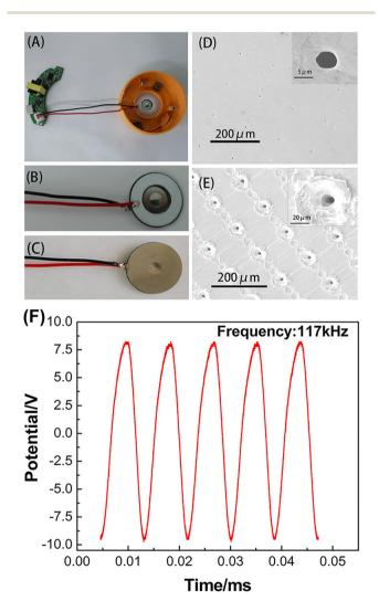
Fig. 13 Schematic representation of an MPUT. (A) The top view of the whole device. Front (B) and back (C) views of the atomizing disc. SEM images of micro-tapered apertures on the front (D) and back (E) sides of the atomizing disc. The insets show the SEM images of a single microtapered aperture. (F) Alternating potential-time profile of the MPUT. Reprinted with permission from ref. 65, Copyright 2020 American Chemical Society.
