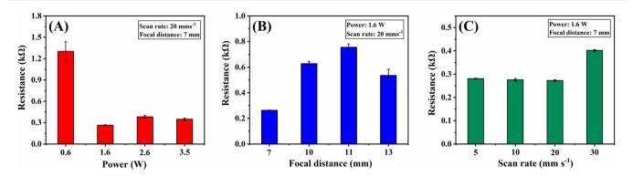
Fig. 2 Effect of IR-laser parameters variation on the electrical resistance of treated 3D-CB/PLA electrodes: (A) IR-laser power (W), (B) focal distance (mm), and (C) beam scan rate (mm  $s^{-1}$ ).
